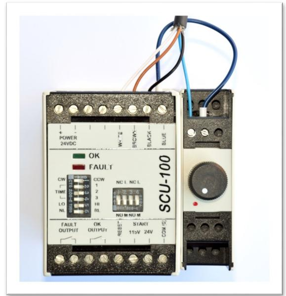
**SCU-100** control unit with **CFR-300** and sensor cable connected
