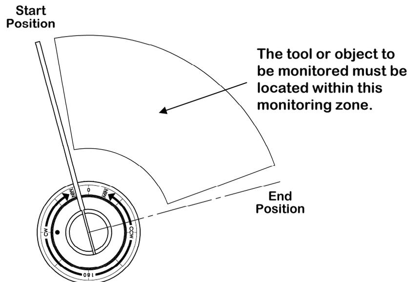
Figure 11: Example of monitoring zone with a 90° CW swing
