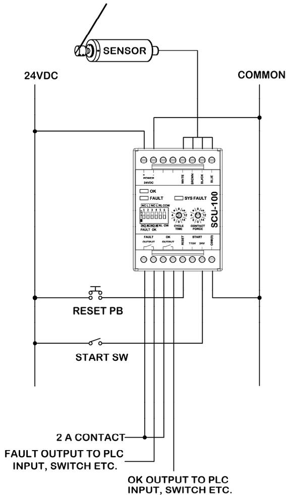
**Figure 14: Wiring diagram (24VDC)**
