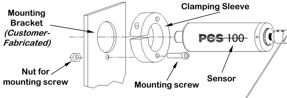
Figure 5: Typical use of Clamping Sleeve
