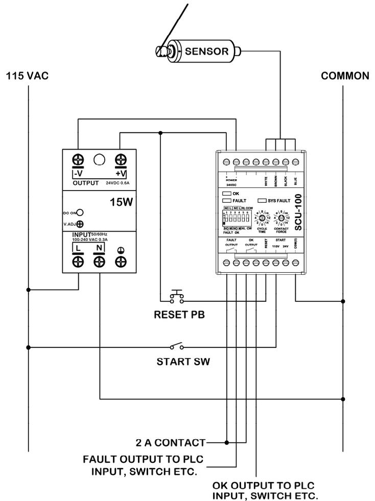
**Figure 15: Wiring diagram (115VAC)**
