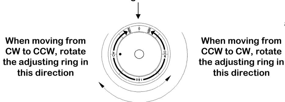
**Figure 9: Adjusting ring movement**
