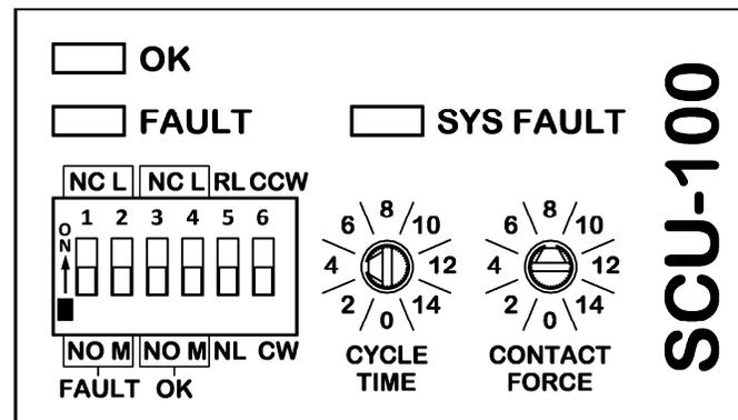
Figure 13: LEDs and switches
