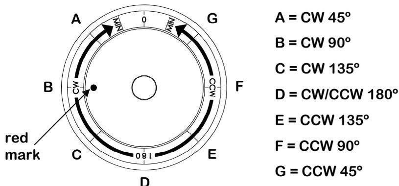
Figure 7: Swing direction and angle selection
